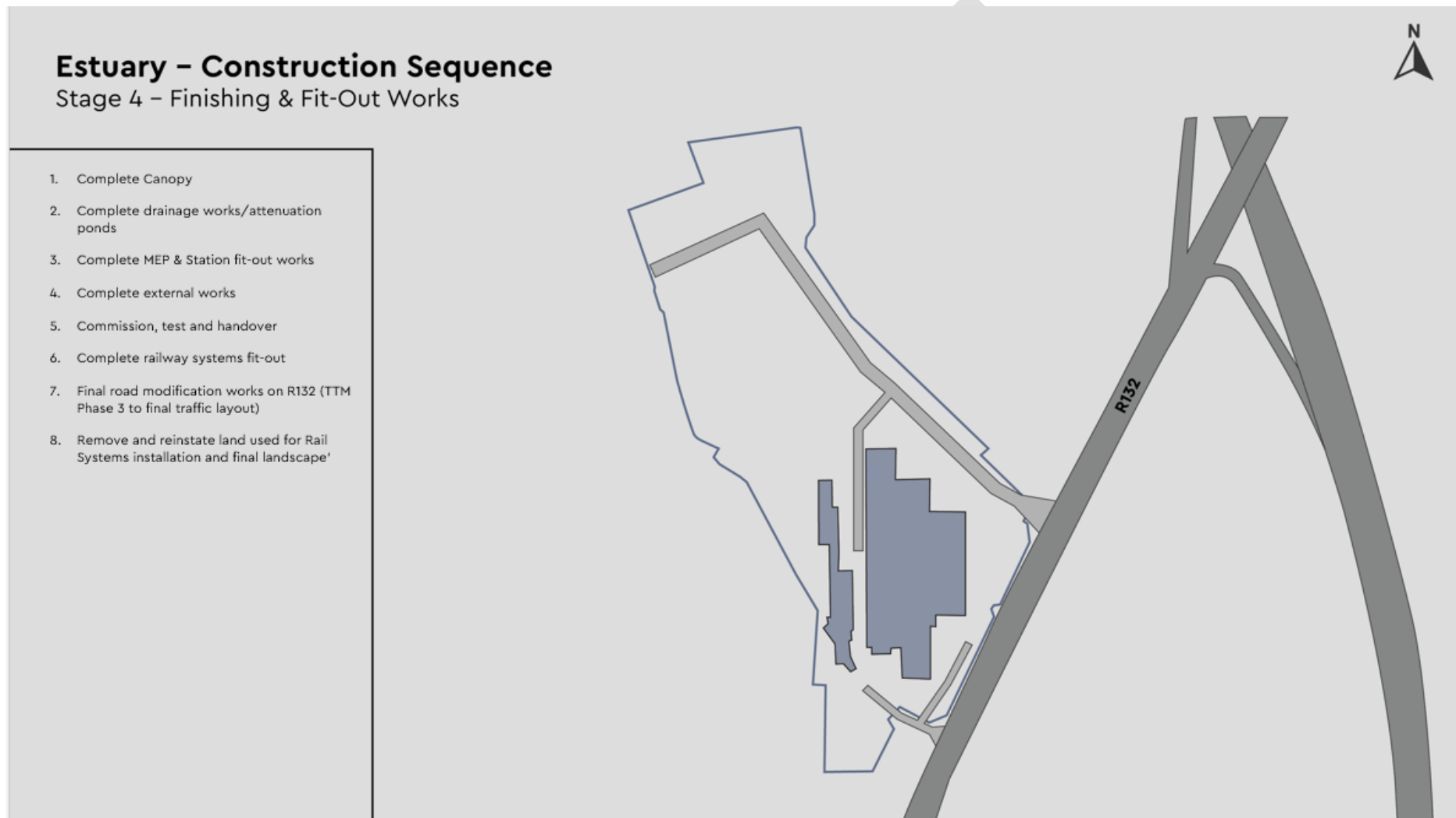
Figure 2-5 Estuary Station - Stage 4 Finishing and Fit Out Works
