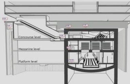
Section B-B, Subway/link & Station
